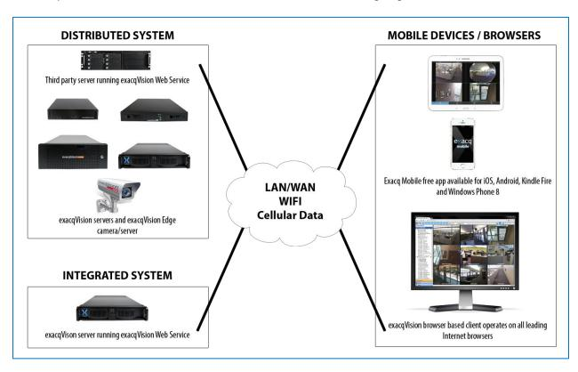
The exacqVision Web Service is normally run as an integrated system on an exacqVision Server. Alternatively, a distributed system with a dedicated web server can be used for higher-capacity systems. Video can be viewed on the local network by using a web browser, over the Internet using a web browser, or on a mobile device using a mobile browser or exacqVision application.
