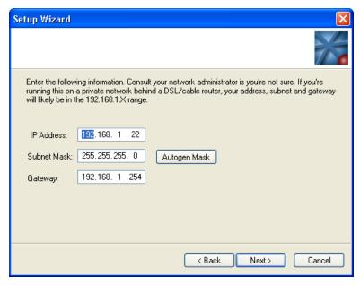
Select either Static IP Address, or Server-Assigned IP Address (DHCP). If you select Static IP Address, enter the IP address, subnet mask, and gateway. Select Only Serve Images on Request, No Upload, Then click Next, and then click Next again to reboot the camera to the new IP address.
