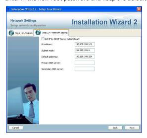
Enter the IP address, subnet mask, default gateway, primary DNS (optional), and secondary DNS server (optional). Select Get IP by DHCP Server Automatically if necessary. Click Next to continue.
