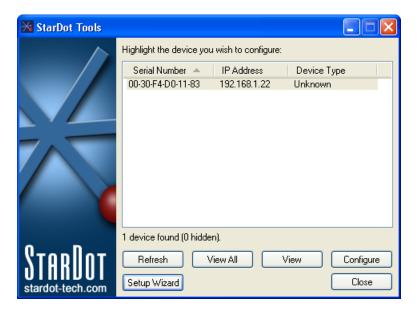
The StarDot Tools utility detects cameras that are on your network. To configure the IP address, select the Camera and then click Setup Wizard.
