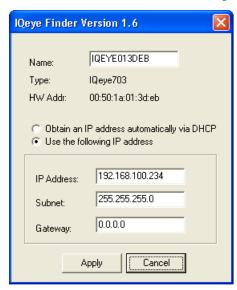
IQinVision cameras typically do not use DHCP by factory default, you must manually assign the camera an IP address. Enter an IP address that is not used by any other device on your local network, ensuring that the first three numbers match the first three numbers of your exacqVision Server's IP address. Set the subnet to 255.255.255.0 and click Apply.
