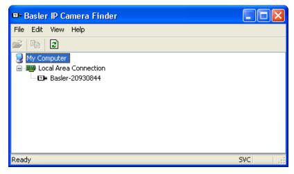
All the Basler IP cameras on the local subnet are displayed under Local Area Connection. To configure a camera, right click and select Open In Browser.
