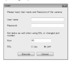
Enter the default credentials and click Execute. When you are logged in, you can assign IP information to the camera. When finished, click Execute. After the camera completes the update, the newly assigned camera information is displayed in the Search results list. **NOTE:** The factory default login for Sanyo cameras is:
