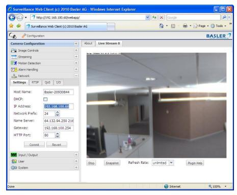
Expand the Network panel to display the camera's Settings tab. Deselect DHCP and then change the IP address and other information as appropriate. Click Commit when finished.
