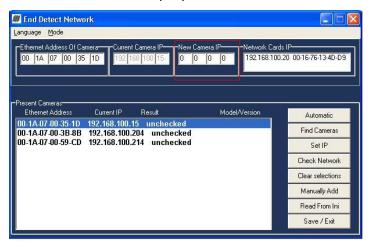
Enter the IP Address in the New Camera IP field.
