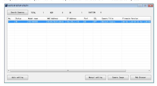
When the camera appears in the Search results list, select the camera and click Auto Setting; this automatically assigns an IP address and other network information to your camera.
