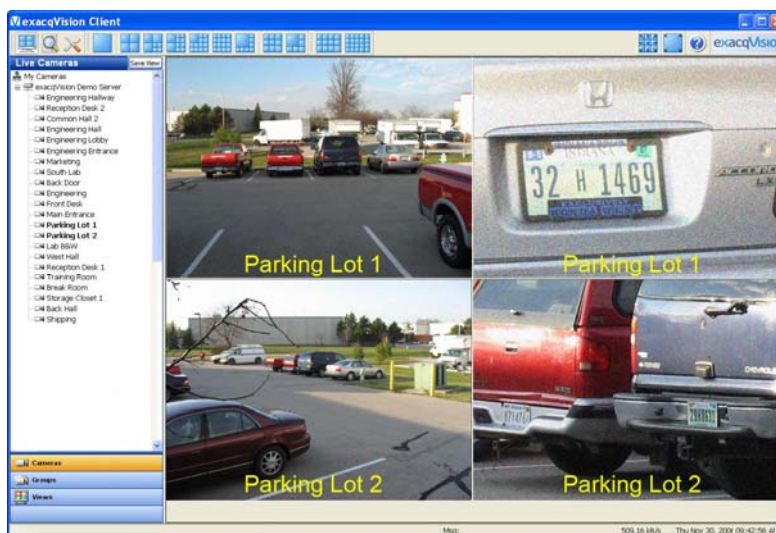
This image shows the “Parking Lot 1” and “Parking Lot 2” megapixel cameras in normal view on the left side of the screen. On the right, these same cameras are opened again and then zoomed in using the exacqVision Digital PTZ feature to reveal greater detail.
